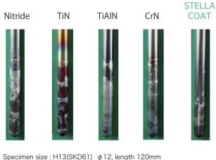
Specimen size : H13(SKD61)  $\phi$  12, length 120mm Aluminum immersion range : 70mm from tip
